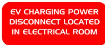
Sign required on a signpost or on the wall directly behind EV charging station.
